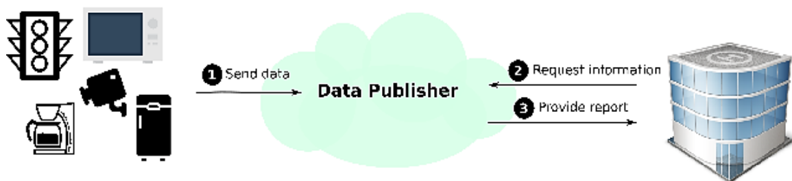
Fig. 3. Generic IoT-centric sensing architecture.
